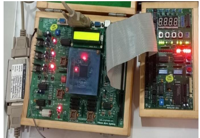
Fig.7. Hardware output using Acex 1K FPGA kit.
