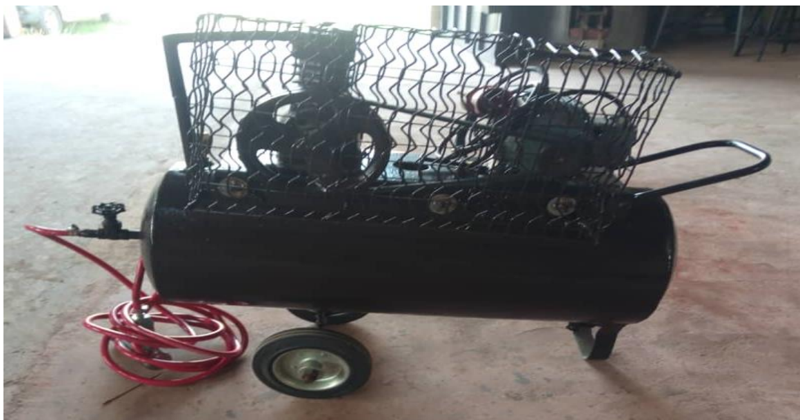
Figure 1: In-house Reciprocating Compressor
