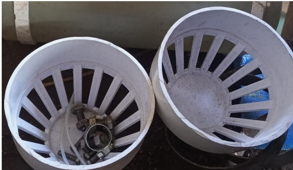
Figure 4: Polyvinyl chloride used as inlet with accessories
