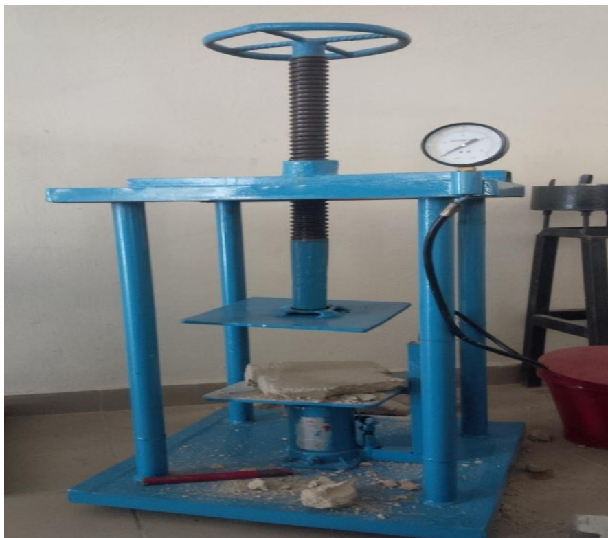
Figure 2: In-house Fabricated Compression Testing Machine
