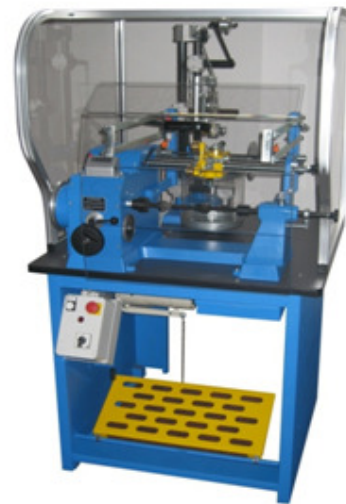
Fig.3. Advanced Semi-Automatic Coil winding machine
