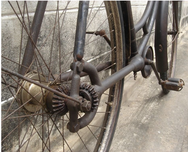
Fig[1].Bicycle operate using shaft drive
