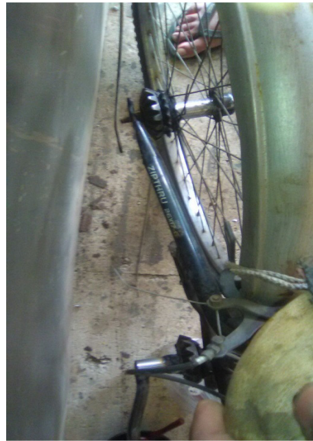
Fig 4 : Placing of Bevel Gear & Drive Shaft
