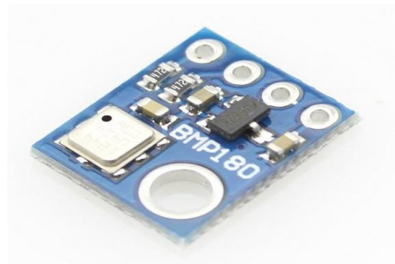
**Fig 5 :** Pressure sensor.
