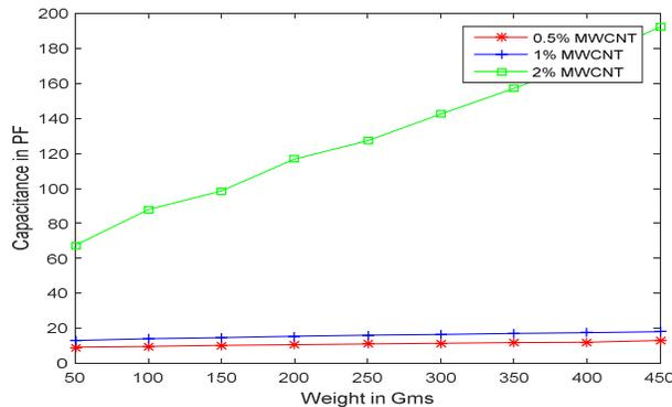
Fig.4. Variation of Capacitance with Weights or stress for different composites of thickness 120 micron at room temperature and at 1 KHz frequency
