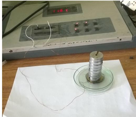
Figure.2 set up to measure capacitance of the samples under different stress conditions
