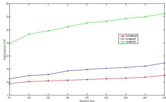
Fig.3.Variation of Capacitance with Weights or stress for different
