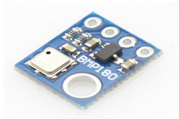
**Fig 5 :**Pressure sensor.
