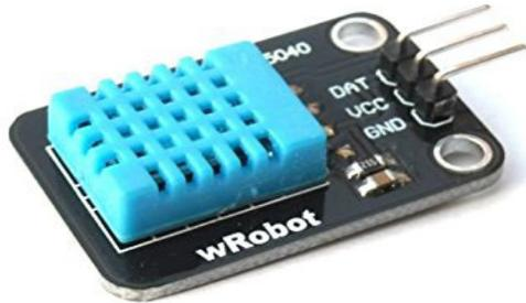
**Fig4:** Temperature and Humidity sensor.
