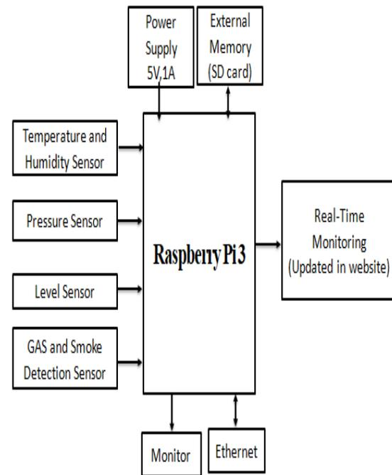
**Fig 1 :**Block diagram of An IOT Based Real-Time Weather monitoring system by using Raspberry pi
