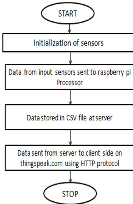
Then the sensors start reading the parameters and the data sent to the raspberry pi 3 then the raspberry process the data and stores in the .csv format then the data is sent to the thingspeak.com by using http protocol the data is finally displayed in the form of graphical representation
