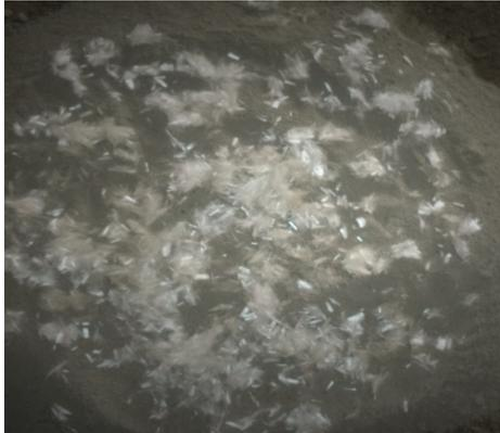
Fig. Mixing of polypropylene in dry mortar
