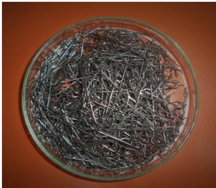
**Fig4.3 Hooked end steel fiber**
