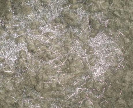
Fig.4.6 Mixing of steel fiber
