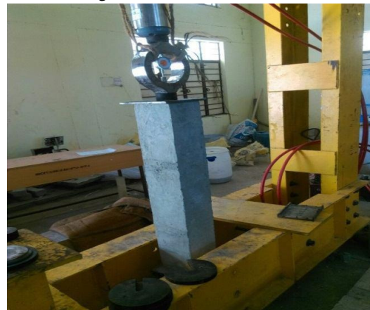
Fig-3: Column Test Setup
