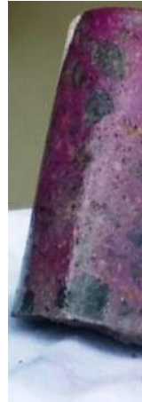
Fig.5.5 OPC core samples subjected to 3 % NaCl
