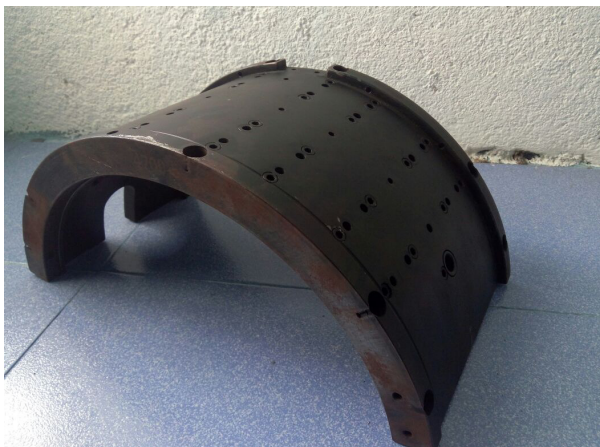
Fig.8 Drill jig manufactured by casting method
