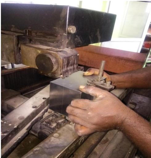
Fig.1 Profile Cutting of MSDM Drill Jig in Wire-cut EDM
