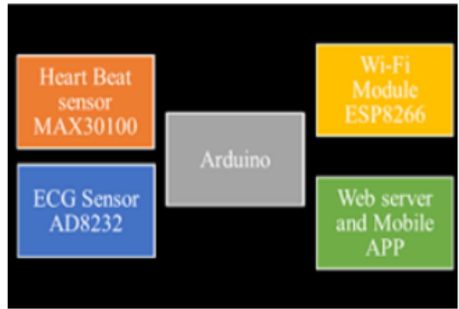
Figure 3: Design of the IOT Device-based ECG System
