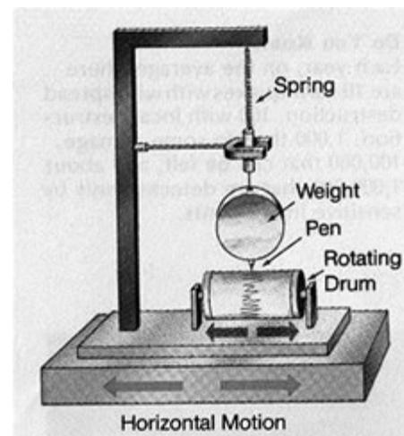
Earthquakes are recorded by instruments called seismographs. The graph output of seismograph is known as seismogram. The seismograph has a base that sets firmly in the ground, and a heavy weight that hangs free. When an earthquake causes the ground to shake, the base of the seismograph shakes too. Instead the spring or string that it is hanging from absorbs all the movement. The difference in positions between the shaking part of the seismograph and the motionless part will be recorded.
