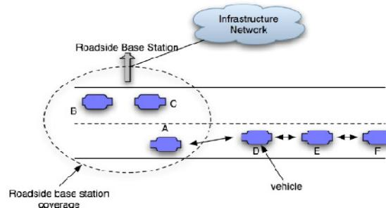
Figure 1: Vehicular network architecture
