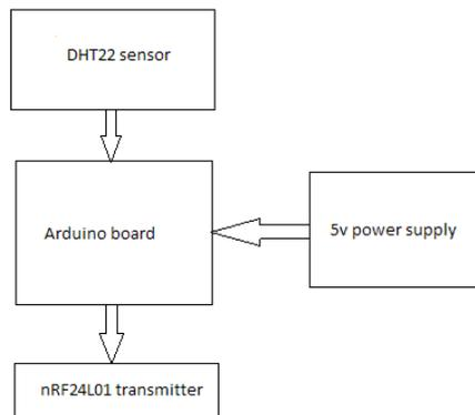
Fig 1. Temperature and humidity data source block diagram.
