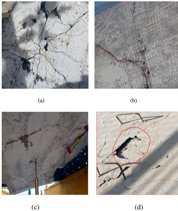
Fig.8 Crack pattern at the face of tested specimens
