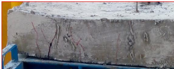
Fig.9 Corner uplift of CON slab
