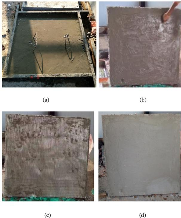
Fig.3 TRM strengthening application steps of specimen C1: (a) Specimen C1 casted (b) first mortar layer application (c) nylon textile application (d) final finished surface
