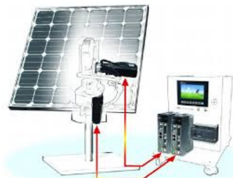
• Fig. 1: Solar tracking system
