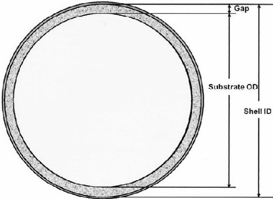
Figure 10: Intersection of Canned Substrate
