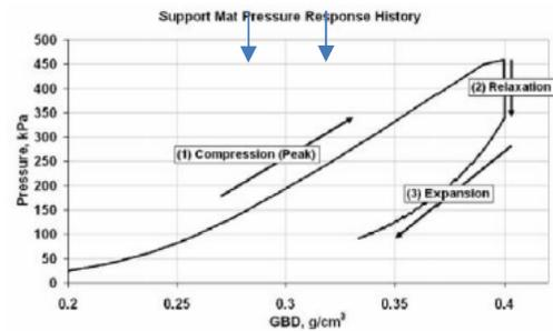
Figure 12: Mat pressure during compression [9]
