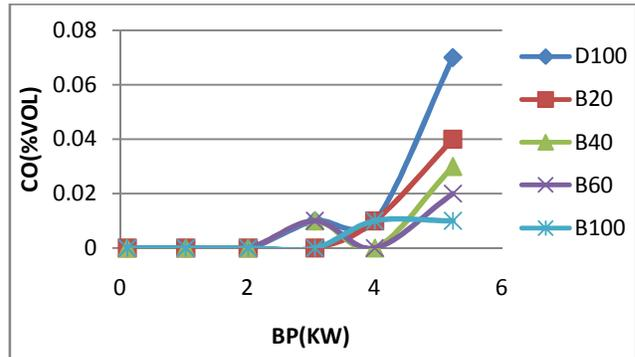
Fig -5(a): Variation of carbon monoxide with brake power without EGR
