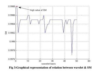
Figure gives relation between wavelet & SM value for different wavelet basis function used in testing. If value of SM is high then that wavelet for which we got high value is best basis.Value of SM should be upto 1.In graph x axis represents wavelet name and y axis represents value of SM.Arrow indicates
