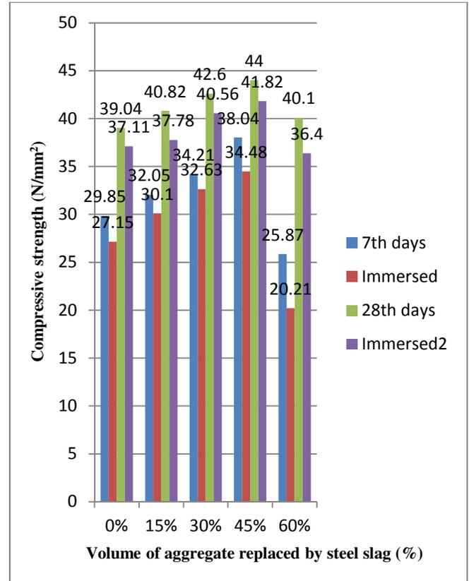
The Resistance to sulphate attack of concrete mix increases upto 16% if 45% of aggregate is replaced by steel slag at 28 days.
