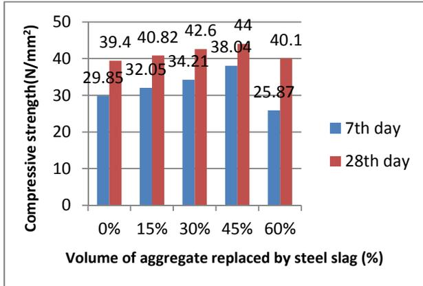
**Fig4.1 Compressive strength of concrete using steel slag at 7th & 28th day**
