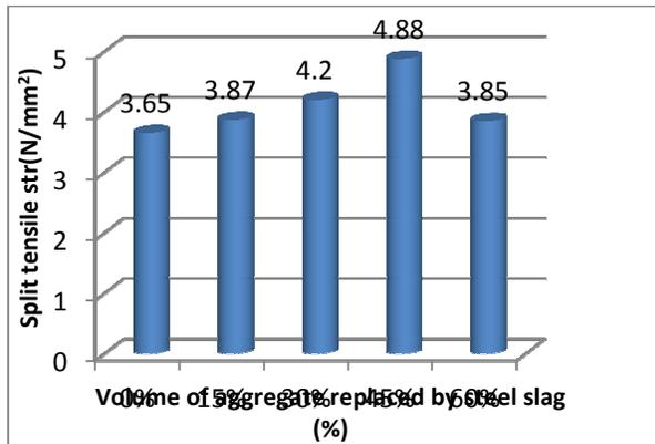
**Fig4.2 Split tensile strength of concrete using steel slag at 28th day**
