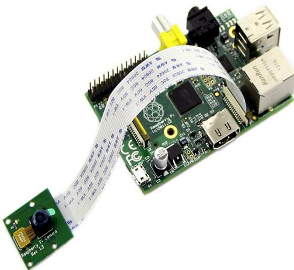
Figure3: Pi Camera Connection on Raspberry Pi
