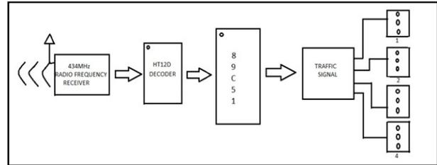
Traffic Signal Controller Block Diagram
