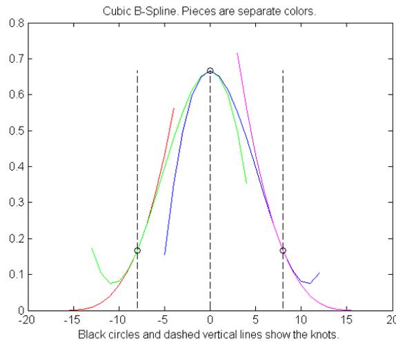
**Figure3. Cubic B-Cline, showing pieces extended beyond the knots.**
