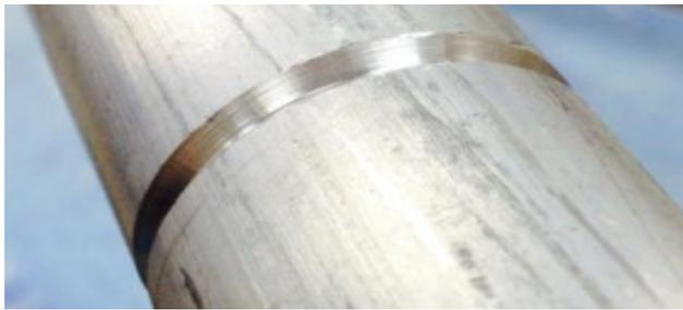
Fig. 1 A picture of a circumferential sharp-notched circular tube
