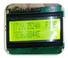
FIG-7 :when fire is detected.
