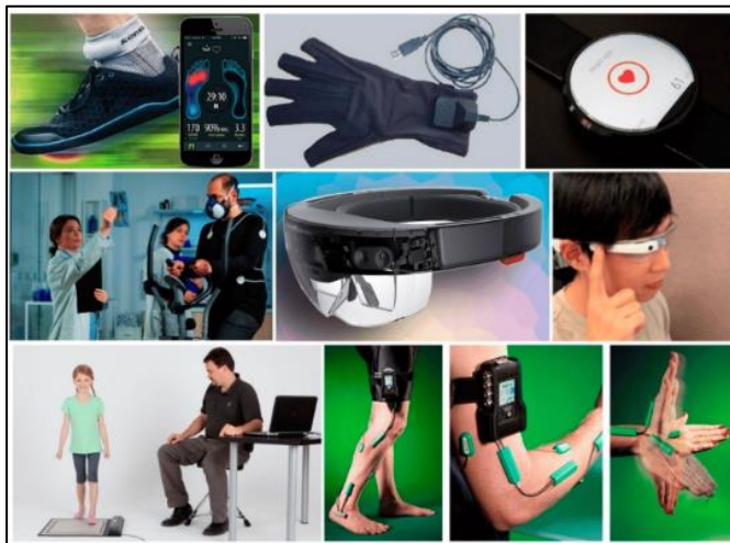
Figure 1 sensors Smart Shoes, Pressure Mats, Leg Sensors, Smartwatches, Head Sensors, Data Gloves, Biometric Goniometers, Torsiometers on Toe and Arm.
