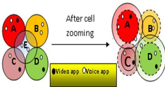
Figure 2.1. Scenario with BS 'E' supporting two voice users and the corresponding optimal network reconfiguration after cell zooming
