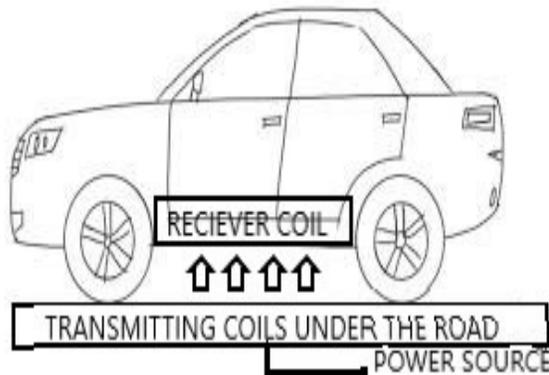
In a following figure it is observed that electric car is fitted with a secondary coil. A set of primary coils are installed inside the road to transmit voltage of 350V at 30kW-hr power. This transmitted power in secondary coil is converted into voltage which is used to store inside a set of Lithium ion batteries. Coils are made up of Copper wire having specified number of turns.
