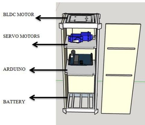
Fig 2 Inner design and component placement
