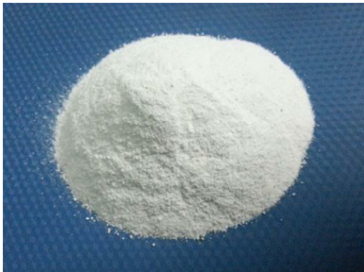
Fig 5: 300µm size glass powder
