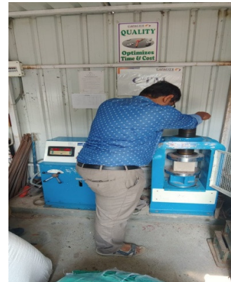
Fig 6: Compressive strength test
