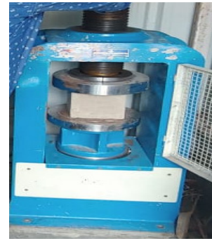
Fig-3 compression testing
