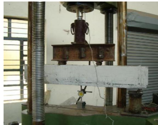
Fig-7 Beam testing process
