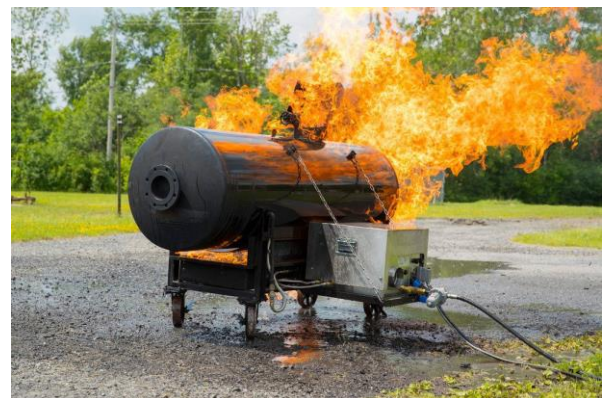
Fig.13. Failure due to excessive temperature
