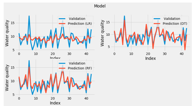
Fig. 2. Comparing the observed and predicted values of the model trained using linear regression, decision tree, random forest
