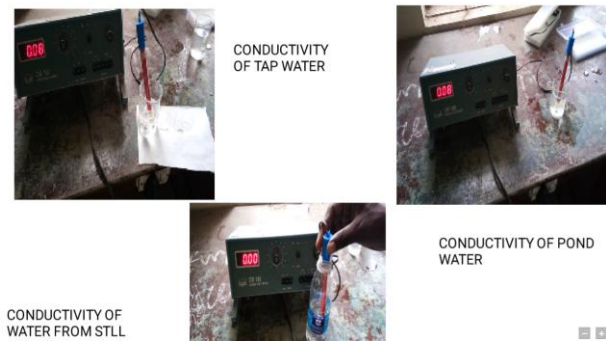
Fig. 4 Example of an image with conductivity check
