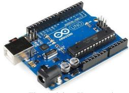
The Arduino Uno can be powered via USB or by an external power supply. The power source is automatically selected. Using pin Mode (), digitalWrite(), and digitalRead(), each of the Uno's 14 digital pins can be used as an input or output.
