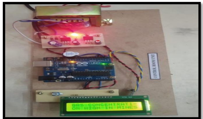
Fig 5: LCD display of Control Room unit, due to MQ-4 Gas sensor
