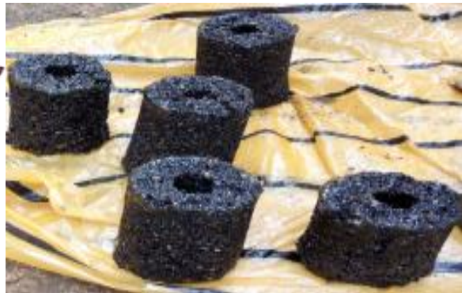
Figure 4: Sun dried produced coarse and fine size briquettes
