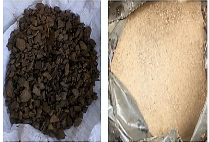
Figure 2: Pulverized and Sieved milled shells
